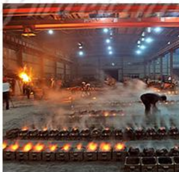
5 pouring and making sand core
